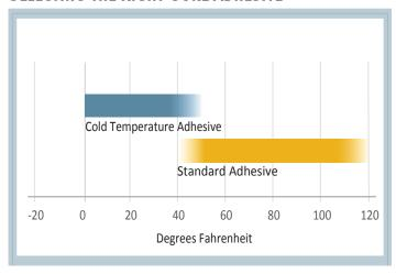
Adhesive range of use may vary based on installation specific conditions including but not limited to surface conditions such as temperature, roughness, and cleanliness including moisture; as well as the specific combination of the Gore Sealant product used and the shape / bend radii of the installation.
